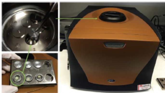
Figure: MultiCell Differential Scanning Calorimeter (TA Instrument). (Photo: UÉVORA)
